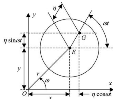
Fig. 5 Geometry of unbalance whirl at the disk
