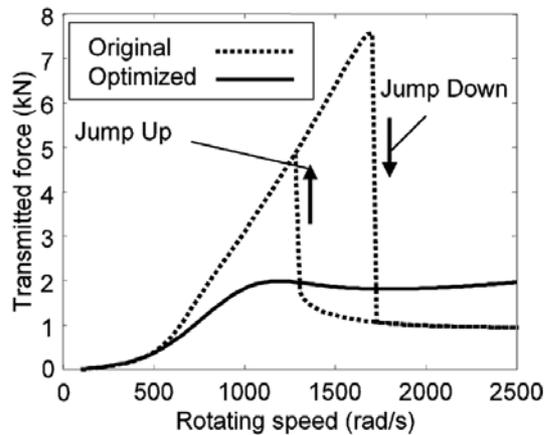
**Fig. 8** Transmitted force for Cases 1, 2 and 3
