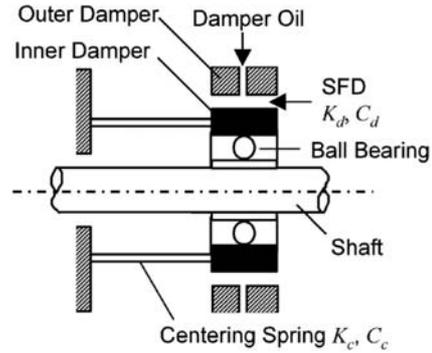
Fig. 1 Typical configuration of a squeeze film damper
